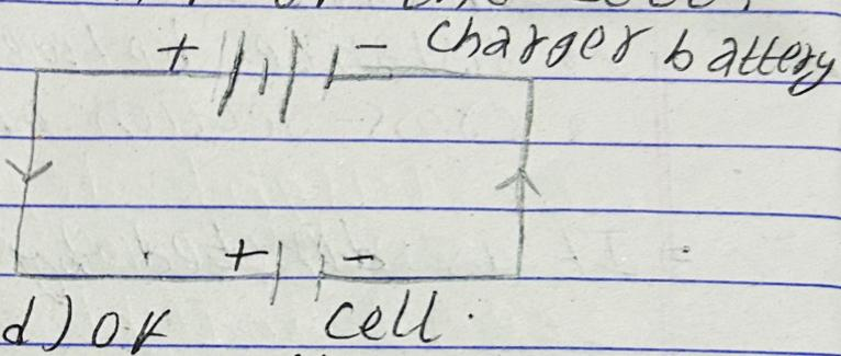
$\Rightarrow$  In charging mode, the +ve terminal of the cell is connected to the +ve terminal of the charger battery and the -ve terminal of the cell is connected to the -ve of the charger battery, so that current is driven by the charger battery through the circuit.
