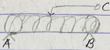
Which is used as a variable resistor and potential divider.
