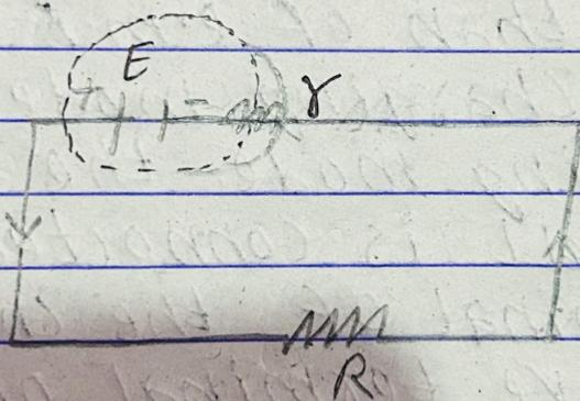
consider a cell of e.m.f.  $E$  and internal resistance,  $r$  is connected to be external resistance,  $R$ . Then, the current flowing through the circuit is given by:
