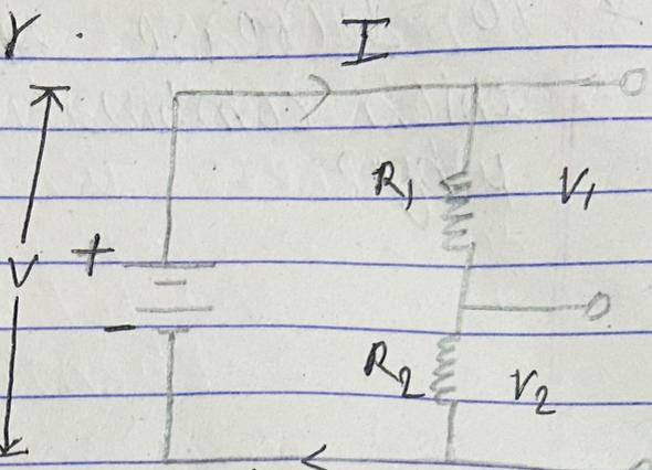
Suppose two resistors of resistance  $R_1$  and  $R_2$  are connected in series through a source of p.d. 'V'. Then current flowing through the circuit is given by.
