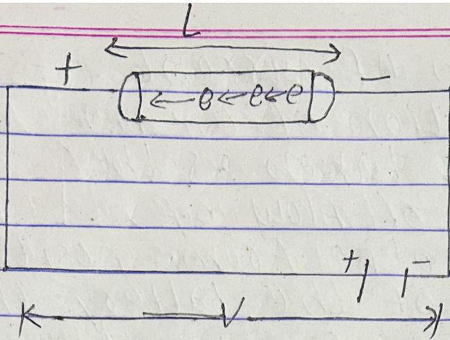
When an electric field is applied across a metallic conductor, the free electrons move from the -ve terminal to the +ve terminal of the battery through the conductor. On their movement, they collide with the +ve ions at which they are retarded. Again between two successive collisions, they are accelerated by the applied electric field.
